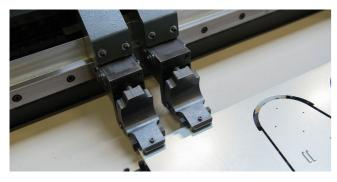
The clamps are set automatically according to the CNC program, minimizing clamp dead zones. When changing production from full size to small sheets, clamps settings can be made automatically without the risk of operator mistakes and without wasting operator time.
