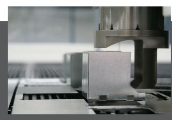
Exceptionally fast forming capabilities. With a bending height of 75mm (3.0 lnches) in a variety of angles and even on parts which are nested in other locations than  $0^{\circ}$  -  $45^{\circ}$  and  $90^{\circ}$  your punch press becomes a multifunctional part processing machine.
