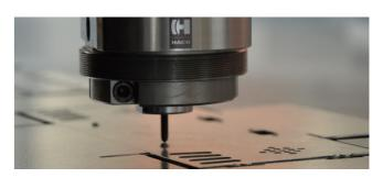
Traditional float tapping or rigid tapping with interpolation, your choice. With the Q series single head punching machines you can use the traditional float tapping system, using a special tap holder. This special float tapping holder will generate the down and up movement for the tap while the C1 axis generating the tap rotation.
