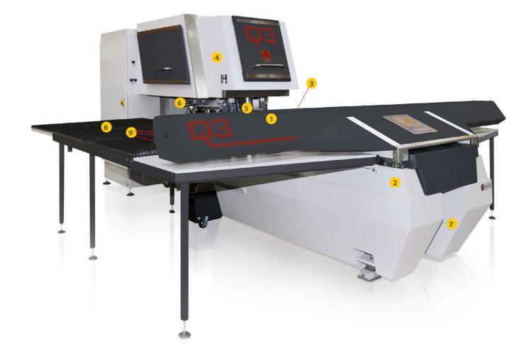
On the large standard brush tables, various workpieces can be nested on standard sheet sizes. The fast AC-servo driven X- and Y-axes with resp. stroke of 2032 by 1524 mm (80" by 60") on Q3 or 2540 by 1524 mm (100" by 60") on Q4 and 3 hydraulic sheet clamps with minimal 'dead zone' 225 by 95 mm (8.85" by 3.74") ensure the highest accuracy on all workpieces (optional CNC programmable).
