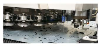
The punch-holder is clamped automatically into the punching head during the tool change. A hydraulic quick-clamping-system is pulling the punch-holder into the punching head, by which the lower part of the punching head (ram) is acting as a mechanical gauge, thus avoiding clearance between punch holder and punching head. While punching, the punch holder and punching head are always connected. The stripper, which is fixed to the punch holder, has two functions:
